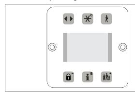
The BDE-D operating unit is an input and output unit for the operation and limited programming of the system. The display shows information about the system by means of symbols and text.
