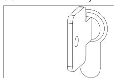
The BDE-Lock key switch is used to lock or unlock the BDE-D control unit for the door.
